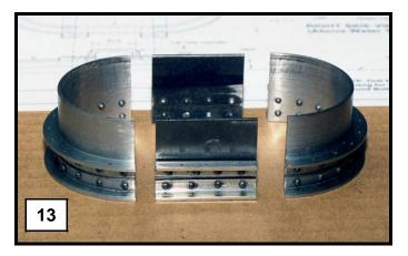
18. Next we will braze together the two Tender Water Tank Funnel ring halves with the streight plates. Prepare the joints by filing a slight chamfer on the inside edges of the joints. To hold these togerther for brazing, wrap a piece of 1/16" diameter welding rod around the outside just below the bottom angle. Hook the ends of the welding rod together tightening for a firm
