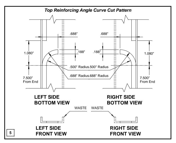
1" x .063" thick wall square steel tube stock and mill the legs to 0.250" wide just as you did in step 4. Each of these reinforcing angles has a row of 27 rivets starting 0.125" in from each end. The remaining 13.000" is then evenly split with 26 spaces at 0.500" center to center. The rivet holes should also be located along the angle 0.094" from the edge of the angle leg or 0.156" from the outside corner. Drill the rivet holes for 1/16" diameter rivets.
